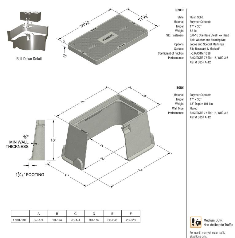
\* Cover comes standard with permanent markings for manufacturer, load rating, model size and manufacturing location.
